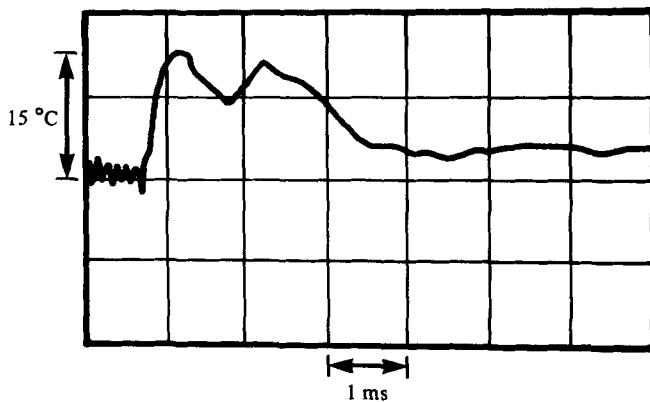
FIGURE 13. Tracing of a typical oscilloscope trace of the interferometer output.
